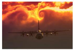
**Wingtip vortices** are circular patterns of rotating air left behind a wing as it generates lift. Note that the vortices are counter rotating
