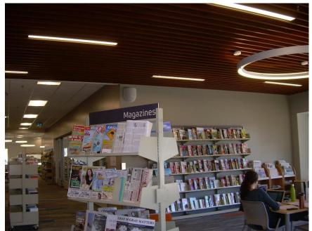
Left, the Quiet Room. The special ceiling panels make this a quiet area. There are no doors but the metal acoustic ceiling eliminates sounds from adjoining areas.
