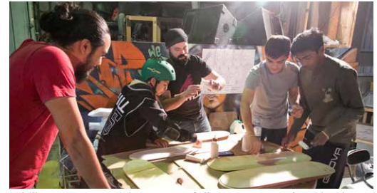
Chill Program participants carefully measure and apply glue to the wooden veneers that will form their own skateboard deck
