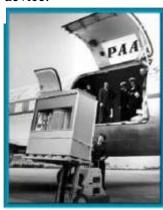
Geoff took us through the history of the hard disc drive, showing the first one: In September 1956 IBM launched the 305 RAMAC, the first computer with a hard disk drive (HDD). The HDD weighed over a ton and stored 5MB of data (see picture left).
