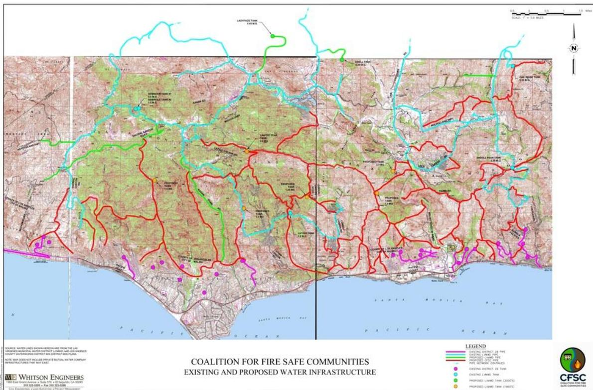
A First Fire Defense is created before fires start by creating a virtual levee and dam system with underground water mains on strategic ridgelines in the Santa Monica Mountains. Prepositioned water distribution points will be put along defensible fire breaks. A sensible system of fire breaks, supplemental water tanks and water mains would be installed.
