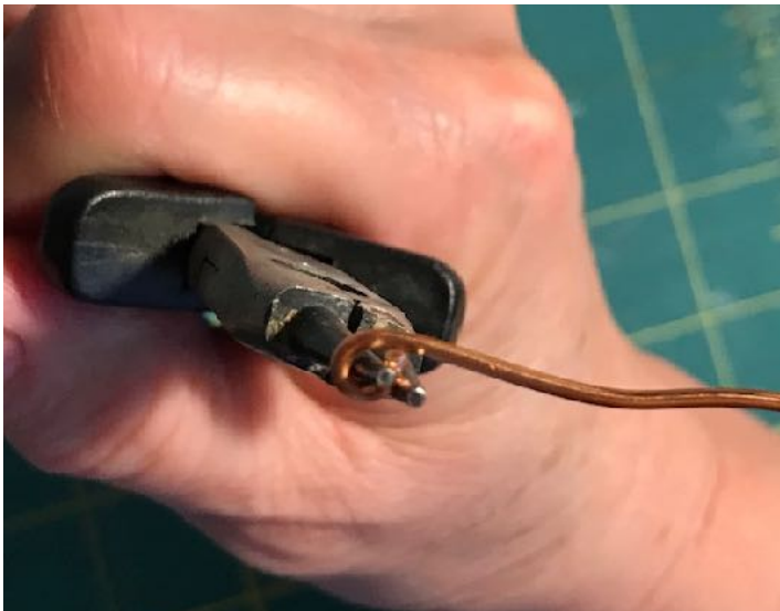
TURN PLIERS UNTIL LOOP TOUCHES THE WIRE
