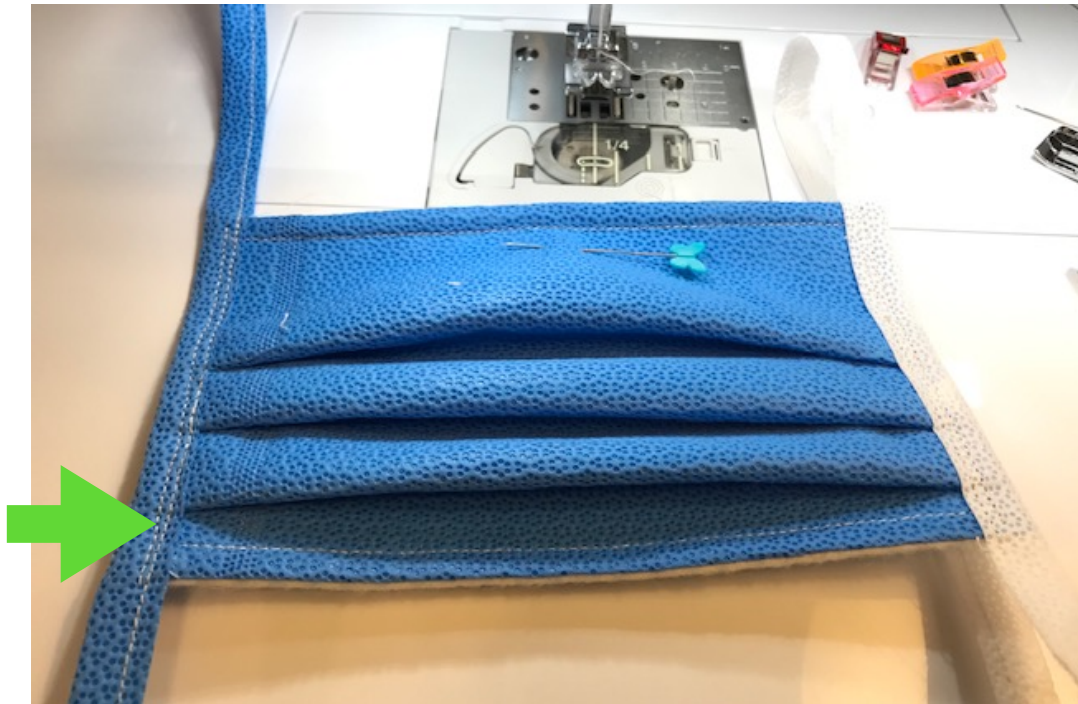
BOTH TIES ON, NOTE 2ND LINE OF STITCHES ON THE SIDE OF THE MASK. ALL FOLDS POINT DOWN AND THE TOP IS WHERE IS SHOULD BE - MY PIN IS AT THE TOP STILL!
