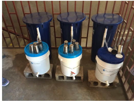
Bio-sand filters in use at a school in Haiti
