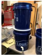
50 filters of the two bucket design were provided. This is the WaterRico design.
