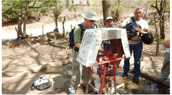
APTU WELL PUMP, LOCATED JUST ABOVE THE STREAM BED
