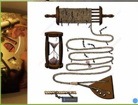
The term **knot** dates from the 17th century, when sailors **measured** the speed of their ship by using a device called a "common log." This device was a coil of rope with uniformly spaced **knots**, attached to a piece of wood shaped like a slice of pie.
