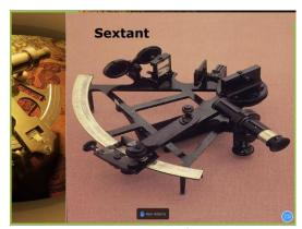
The sextant is a doubly reflecting navigation instrument that measures the angular distance between two visible objects. The primary use of a sextant is to measure the angle between
