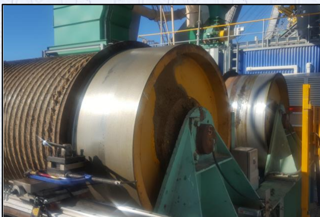
The completed drum after machining.
