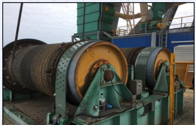
Completed job with new brake-shoes in place.
