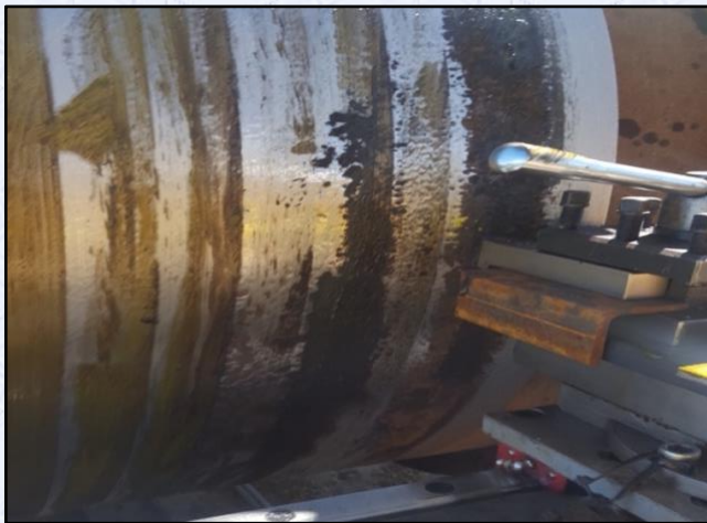
The completed drum after machining.
