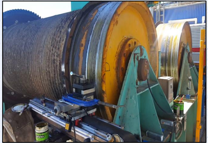
Completed job with new brake-shoes in place.
