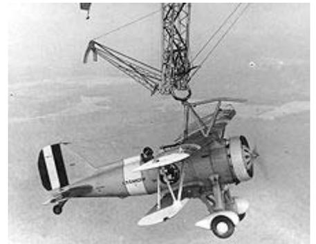
The really tricky part was getting the planes back onto the airship. Each plane had a large hook mounted on the top wing; the pilot had to snag a large hoop on the trapeze with his hook and quickly kill the engine. The precursor to today's tailhook?
