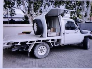
Figure 92: The canopy mounted to the ute with its doors open.
