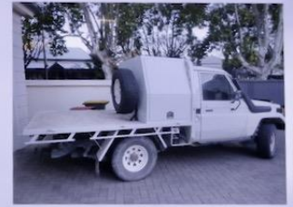
Figure 93: The canopy mounted to the ute with its doors closed.
