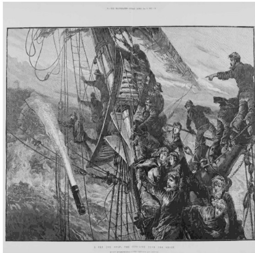
ABOVE: A Cry for Help the Life Line from the Shore. A Cry for Help, the Life-Line from the Shore, Rocket Apparatus used by the Volunteer Life Brigade. Illustration for The Illustrated London News, 8 January 1837. The volunteers used a 'Rocket Life-saving Boxer' to fire a line over a stricken ship. The line had a heavier rope with a tail-block and pulley attached. This was secured to the ship and a breeches buoy, which could then be hauled between the ship and the safety of the shore.
