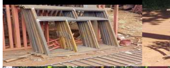
MAKING STEEL WINDOWS FOR RENNOVATION OF TEACHER'S HOUSE AT MAMBA SCHOOL (WELDING)
