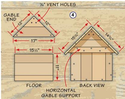
4. Glue and screw the gable ends to the supports. Screw the roof cleat to the inside of the gable ends. Glue and screw the roof in place. Drill two 1/4" holes at the top of each gable end for ventilation.
