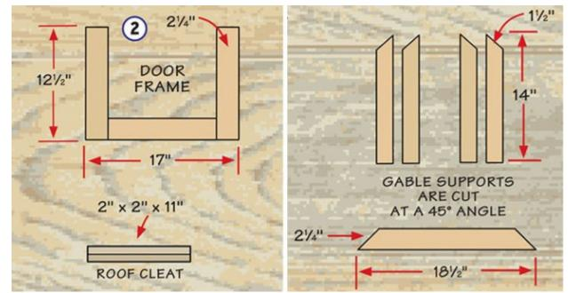
3. Use the drawings as a guide to cut to size the roof, walls, floor and gable end sections. Glue and screw the walls, floor, door frame and gable end supports together.
