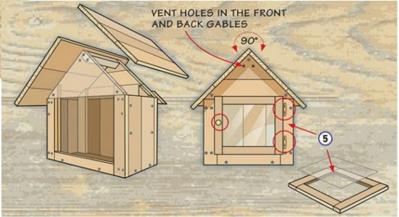
Before assembling, paint all pieces except for surfaces to be glued. Use oil-based rust paint to protect against weathering or any high quality oil-based external paint.
