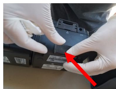
Replacing the air intake filter
