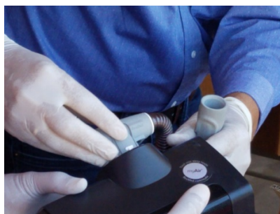
Removing ventilation tube & attachments
