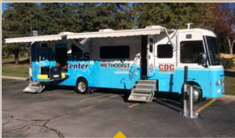
View with retractable steps, wheelchair lift, roll-out awnings
