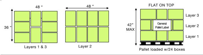
**Placard the pallet** on all four sides with General Pallet 11" x 8.5" Content Description labels (these can be downloaded for the Tool Box web-page)
