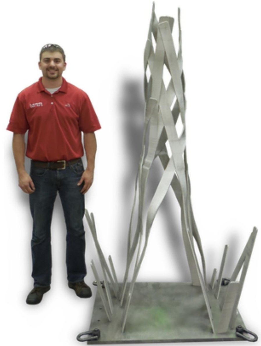
Ti-6Al-4V Structure - 7ft Tall
